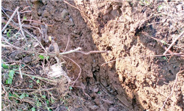
PLATE 10: Test Pit 1: Detail of test pit showing glacial sub-soil consisting of clean, pink boulder clay overlain by a layer of light brown clay mixed with small stones.
